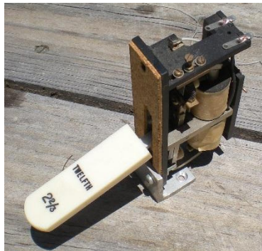
All Kimber Allen console stop tab switches are fitted with set/reset coils
