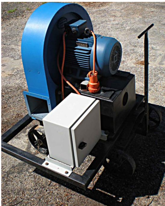
Three images of restored blower unit mounted on mobile trolley and equipped with new 3-Phase motor & soft-start controller enclosure
