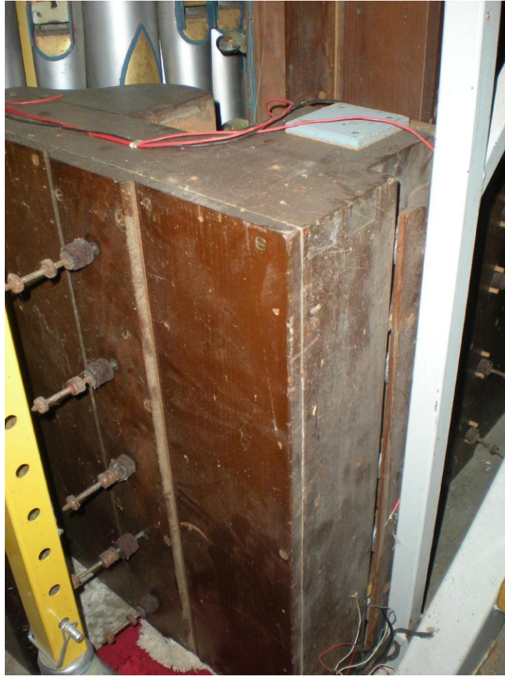
Original Dodd pneumatic actuators
