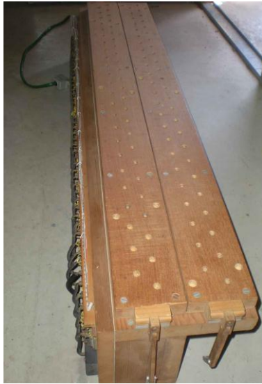
Bar & Slider unit intended to be used in floating Choir division – uses Kimber Allen electro-pneumatics
