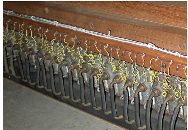
Bar & Slider unit intended to be used in floating Choir division – uses Kimber Allen electro-pneumatics
