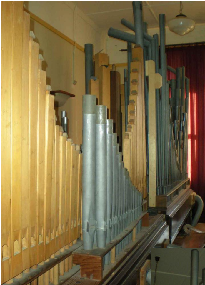
Front left view of Great & Swell divisions. The foreground metal pipes are the Great Diapason upper octaves, with the stopped wood Lieblich Gedact immediately behind
