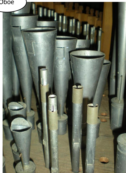
Highest four notes in the Oboe rank are flue pipes
