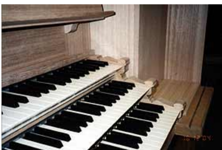
The newly reconstructed Hill & Son console, showing the new three manual key sets by P&S, and surrounds by John Stephens.
